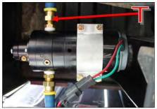
C. Route suction line to port 'T'. Cut FL-1002 to needed length and connect to 10-300 in port 'T' using the PL-1005. Be sure to oil both before attaching.
