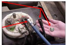
NOTE: Hose clamps are not recommended for push lock fittings. They will hold up to 300psi! Use oil on fittings and inside fuel line when installing Push-Lok fittings
