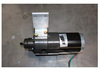
C. Using thread tape, install the 2 10-300 into the "T" & "E" ports. Torque to 40 ft./lbs. Connect the male end of the wire harness to the female electrical connector on the FASS pump. Reconnect the battery. Turn key to the "On" position. With the FASS pump on, squirt a liberal amount of WD-40 or other lubricant into the "T" port. This procedure will "wet" the Gerotor and allow for better suction during initial priming. **Note: Do Not Put Thread Tape on Flare of Fitting**
