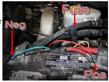
D. Secure relay and fuse in an upright position, as shown, to prevent moisture from entering. Di-electric grease may be applied to prevent corrosion.
