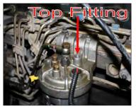
F. Measure and cut fuel line. Insert PL-2003 90° Push-Lok fitting using oil. Install fitting to DIPF-1003. Torque to 18 ft/lbs.
