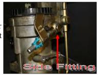
F. Measure and cut fuel line. Insert PL-2003 90° Push-Lok fitting using oil. Install fitting to DIPF-1003. Torque to 18 ft/lbs.
