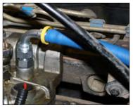
Note: Secure all fuel lines with cable ties. Cable ties are an economical way to prevent the possibility of problems occurring!
