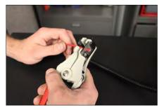
B. Place wire from 46044 and WH-1006-3 into butt connector. Using crimping tool connect 46044 and WH-1006-3 with butt connector. Install 46260 to 46044 top slot (opening that is near the spade). Route Add-a-fuse lead through the fire wall using existing grommet. The use of corrosion preventative spray is recommended.
