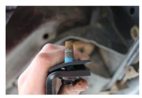
B. Secure FAB-1001 onto the FA assembly with supplied 1/4-20x0.75 bolts.
