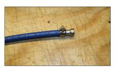
B. Disconnect factory suction line clip by pressing in on the two tabs located on either side in the connection fitting. Once removed, clean the suction tube and connect the QD-1002 addressed in the previous step. Bed is removed for photo clarity.
